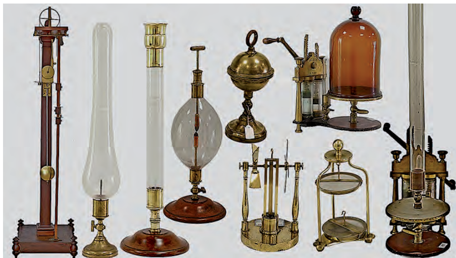
Fig. 4. Some Deleuil's scientific instruments purchased by E. Taranto Rosso in Paris in 1846. From left to right: Atwood machine, fountain in a vacuum, mercury shower, electric egg, double windmill, Magdeburg hemispheres and adhesion plates, double barreled air pump, Guinea and Feather tube
