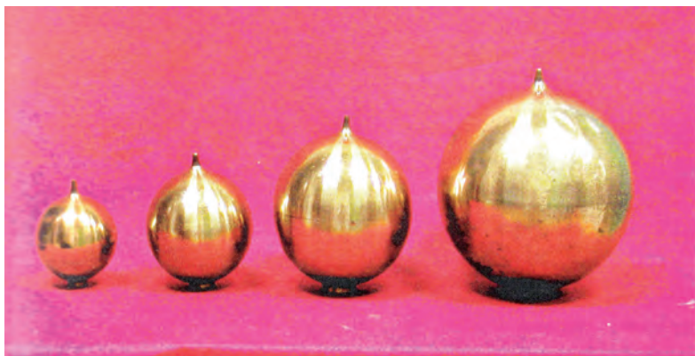
Fig. 1. Helmholtz resonators. Used to amplify and perceive a specific note. The larger (lower) opening kept contact with outer air; the smaller, on top, had a shape adequate to insert it in the experimenter's ear
