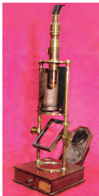
Fig. 3. Norremberg polariscope. It is a polariscope with an Amici microscope; these instruments allow to measure crystals with a beam of light polarized at will
