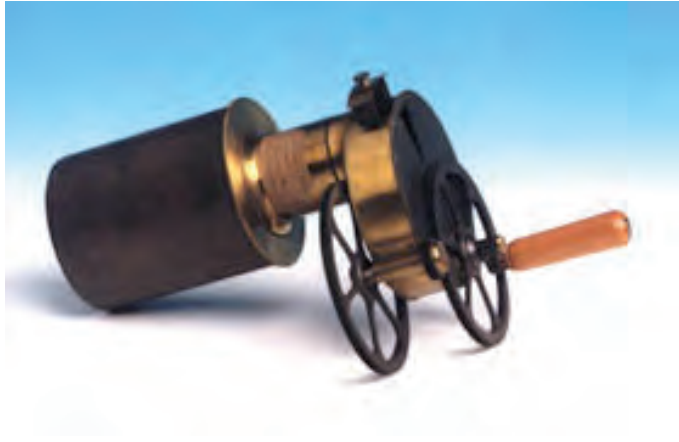
Fig. 4. Becquerel phosphoroscope. It measures whether a substance is, or is not, phosphorescent, even for a short time
