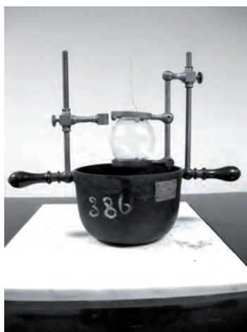
Fig. 2. Dumas apparatus for the determination of vapour densities (Museum of Chemistry, University of Palermo)
